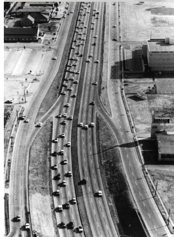
Central Expressway, Dallas at the peak of traffic in 1958. The estimated hourly traffic load per inside lane was better than 2,000 vehicles per lane, per hour. (courtesy of TxDOT)
